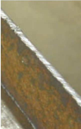
The plasma cutter leaves a striated edge on the steel similar to that of an acetylene torch. It requires some dressing with a grinder to create a finished face.
