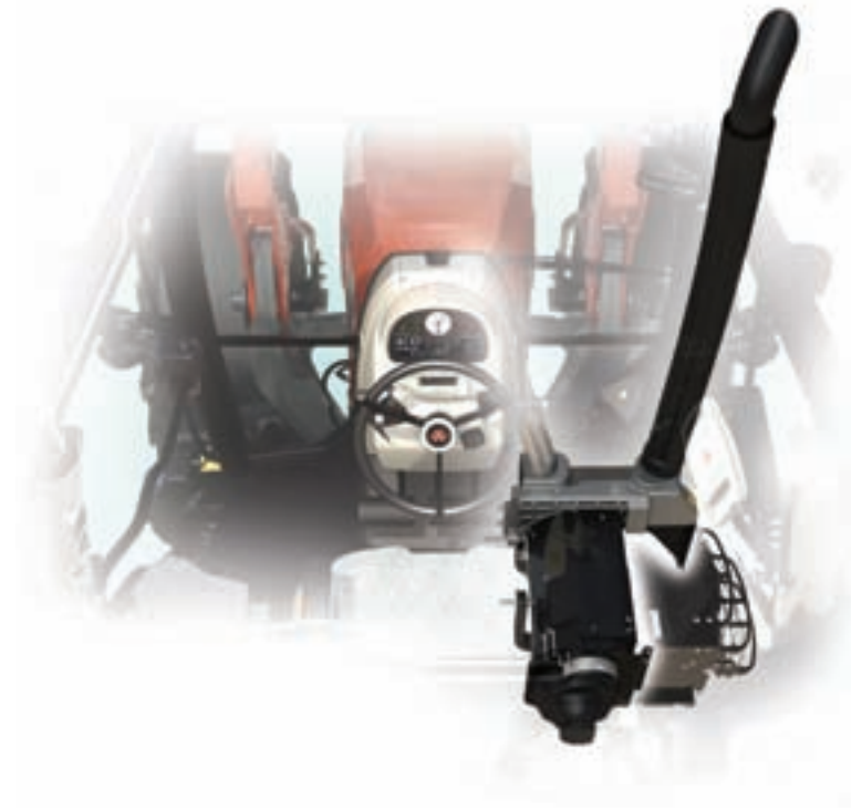
The compact size of the All-In-One SCR emissions treatment system allows it to be mounted under the cab on the MF 5713 SL.
