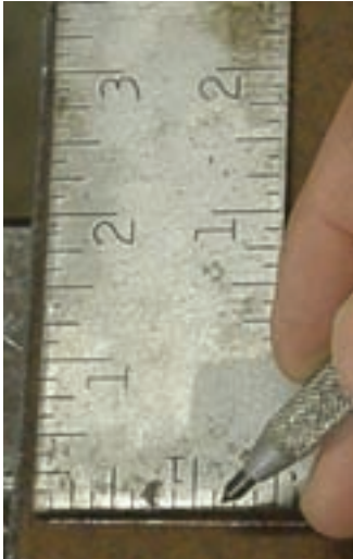
Using a scribe to mark cut lines allows for transferring precise measurements and exactly positioning the torch guide.
