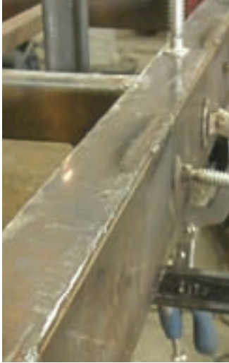
Welding was spread out along the length of the joint to prevent concentrating heat into one area and warping the metal.
