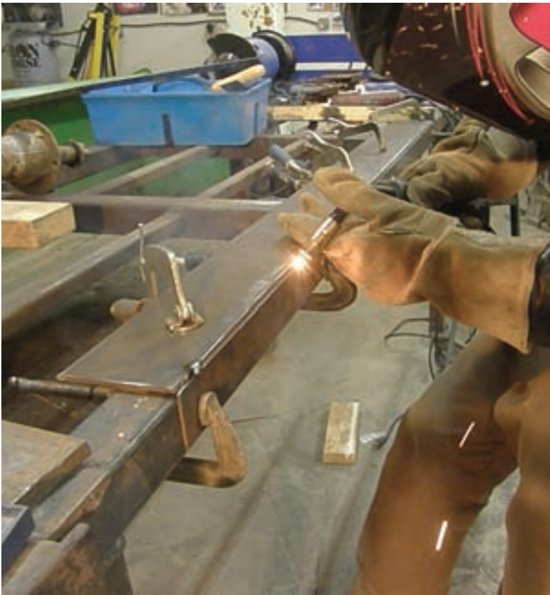
Clamped firmly in place, the two pieces of steel forming this 90 degree outside joint are positioned properly, allowing for excellent weld penetration.
