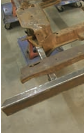
Fitted into place with the original bent and broken part behind it, the replacement bumper looks exactly like the original once did. The only thing left to do is drill holes for the mounting bolts.
