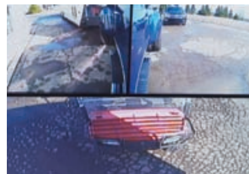
Top: GM will offer a retrofit camera package for 2014 to 2016 Silverado trucks to make trailer towing easier and safer. Left Bottom: Side rear-view cameras get integrated into the Silverado side mirrors. Right Bottom: Camera views appear on the centre dash screen in the truck.
