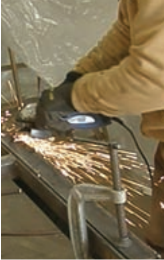
An angle grinder is used to smoothen out the weld bead and make the bumper look like one seamless piece.
