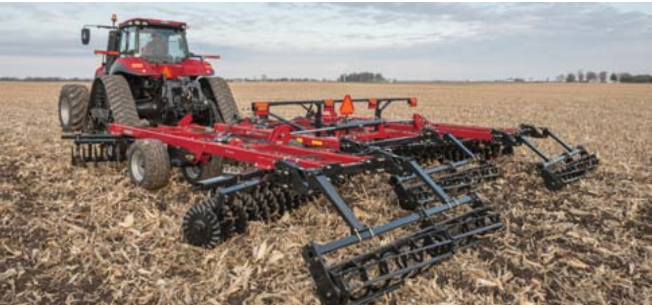
Left: New from Case IH is the True Tandem 335 Barracuda vertical tillage tool for aggressive field finishing. Top Right: The Barracuda uses 22-inch serrated blade design.
