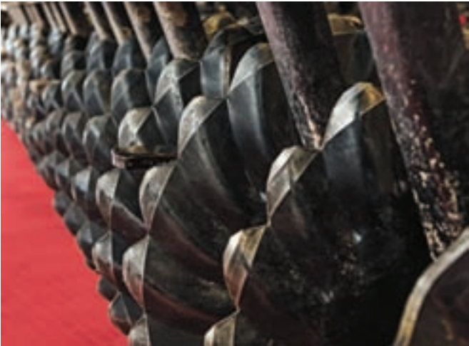
Left: New from Case IH is the True Tandem 335 Barracuda vertical tillage tool for aggressive field finishing. Top Right: The Barracuda uses 22-inch serrated blade design.
