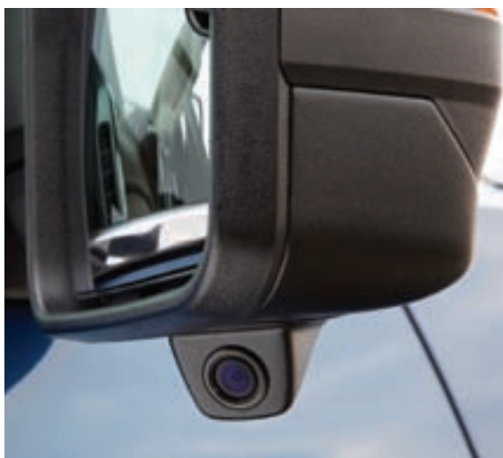
Top: GM will offer a retrofit camera package for 2014 to 2016 Silverado trucks to make trailer towing easier and safer. Left Bottom: Side rear-view cameras get integrated into the Silverado side mirrors. Right Bottom: Camera views appear on the centre dash screen in the truck.
