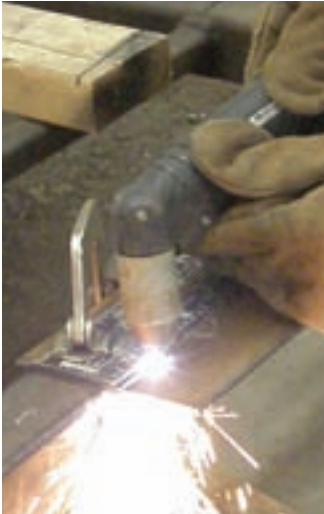
A framing square was used as a guide for the plasma torch to ensure a perfectly straight edge.
