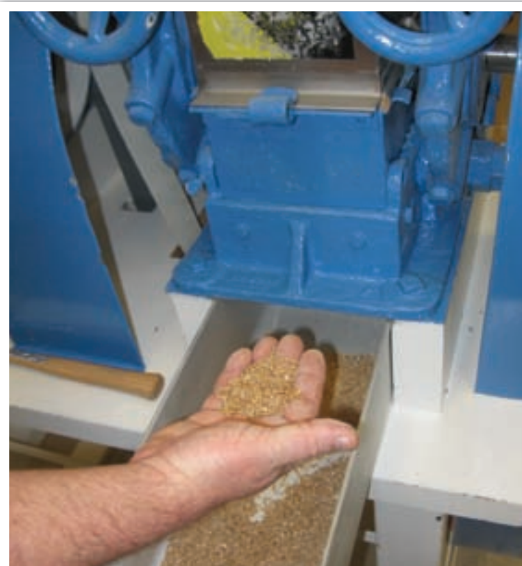
Allis Chalmers roll stands in the CGC lab have been in use for at least 80 years.
